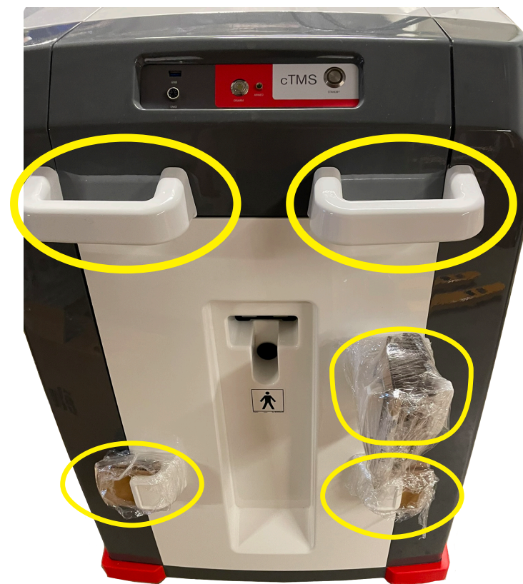
Fig. 2-4 Main chassis with locations of protective spacers indicated in yellow
